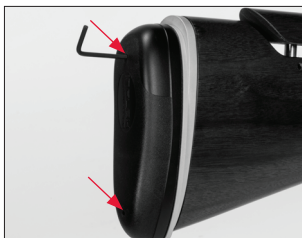
Locate and carefully remove the screws that secure the recoil pad to the pad plate.
